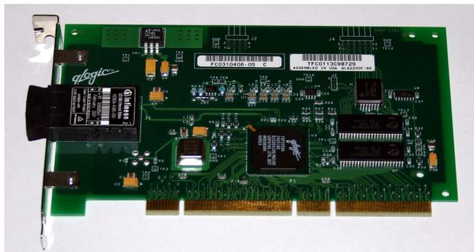
FIGURE 2.26 – Host Bus Adapter Fibre Channel
