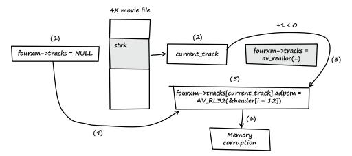
Figure 4-3: Unexpected behavior of FFmpeg causing memory corruption
