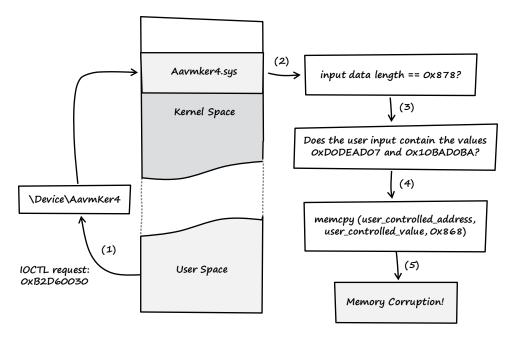
Figure 6-6: Overview of the vulnerability from IOCTL request to memory corruption
