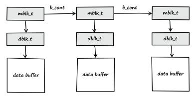
Figure 3-2: Diagram of linked STREAMS message blocks
