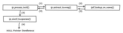
**Figure 3-4:** Call graph summarizing the relationships of the functions involved in the NULL pointer dereference bug. The numbers shown refer to the chronological order of events.
