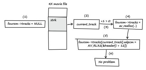
Figure 4-2: Expected behavior when FFmpeg operates normally
