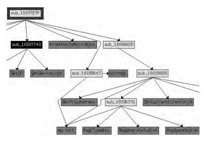
Figure 5-8: Code path to reach the vulnerable function (created in IDA Pro)
